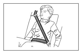
4. Buckle, position, and release the safety belt as described in *Rear Seat Passengers on page 31*. Make sure that the shoulder belt crosses the shoulder.
